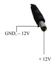
Jack plug connection when using an external power supply unit 12V DC/60W power supply
